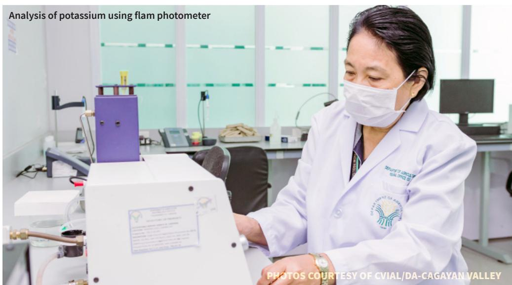
Analysis of potassium using flam photometer
